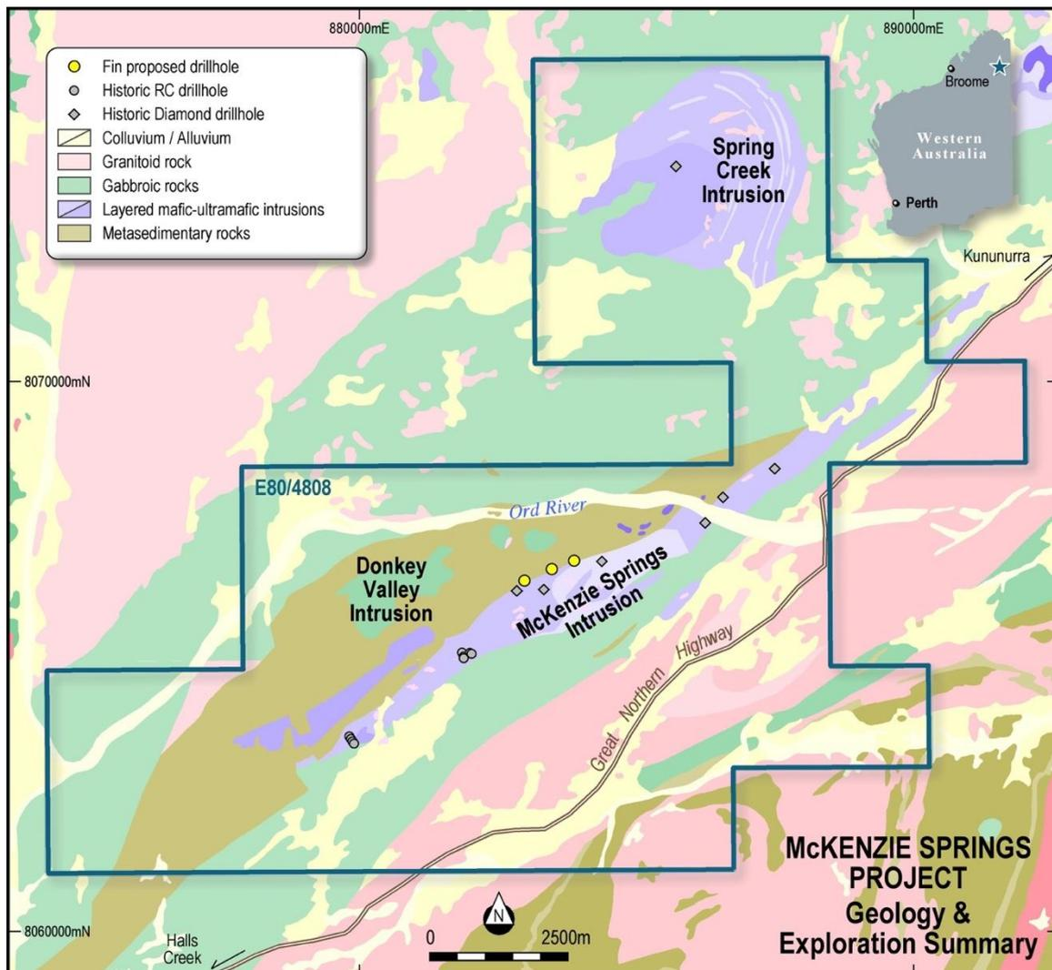
Figure 3: McKenzie Springs Project geology, existing drillholes and proposed diamond drillholes
