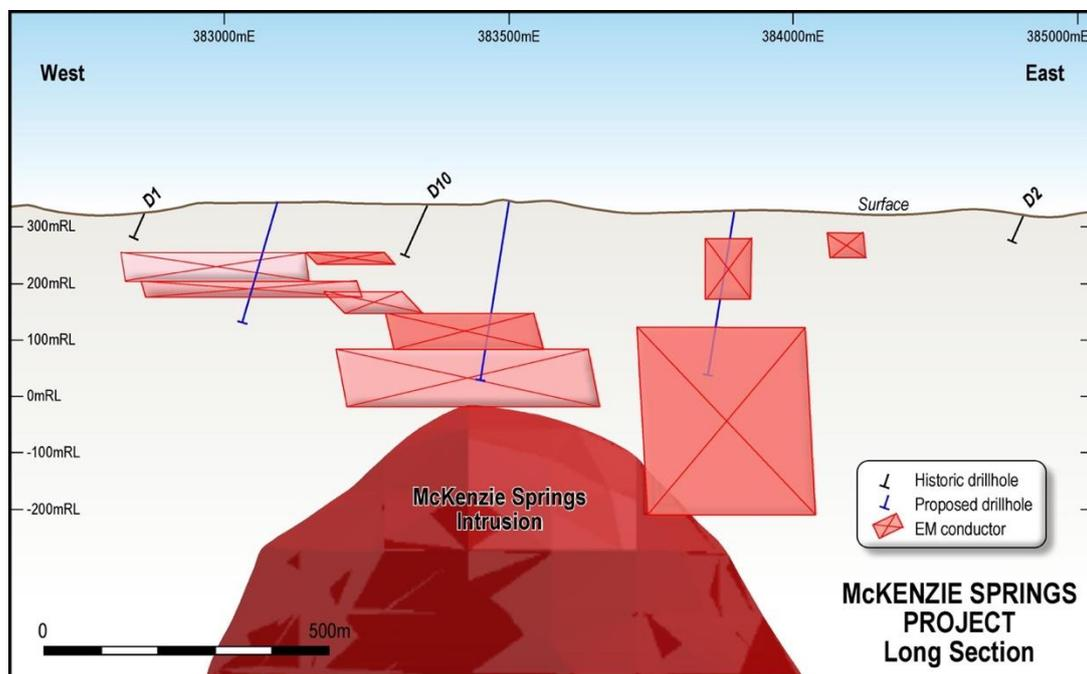
Figure 2: Interpreted model of the McKenzie Springs intrusion, FLEM plate models, existing drilling and proposed drillholes.
