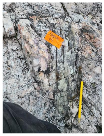
Figure 2 | Large green spodumene crystal with fine lepidolite near left crystal margin
